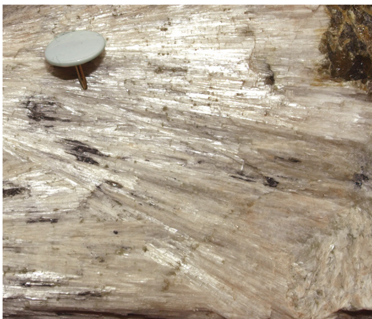
Figure 3 Contact-metamorphic off-white wollastonite with small amounts of manganese causing a brownish hue. Location: Kimeria, N Greece (Photo Rob Hellingwerf)
