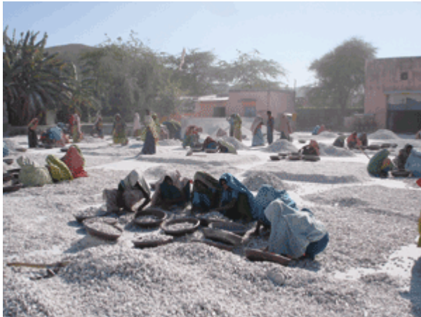
Figure 12 Hand sorting of wollastonite at Wolkem's facility near Udaipur, Rajasthan
