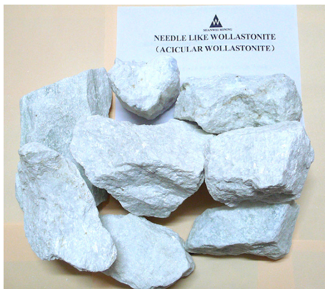
Figure 7 Wollastonite pieces from a Chinese producer (Photo Jilin Shanwei Wollastonite Mining Co., LTD).
