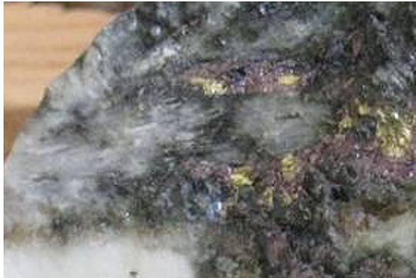
Figure 4 Contact-metamorphic wollastonite accompanied by a.o. purplish bornite and yellow chalcopyrite. Location: Demirtepe, Turkey. (Photo Empire Mining Corporation)
