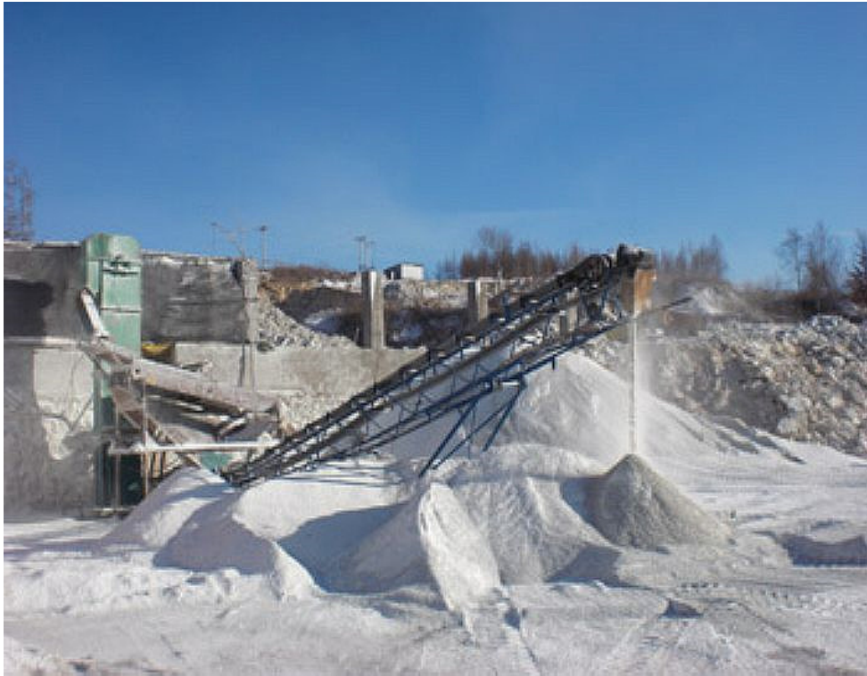
Figure 10 In-pit crushing of wollastonite (Photo Jilin Shanwei Wollastonite Mining Co., LTD).
